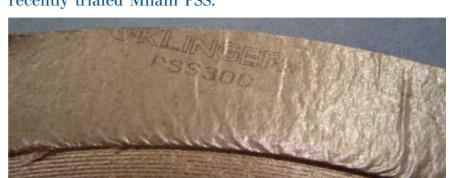
The spent gaskets (pictured) showed no signs of deterioration caused by media or high temperature and were acclaimed by mechanical staff for their ease of removal. Milam has also proved to be a robust material resistant to the ill effects of manual handling. The customer was said to be impressed by Milam's quality of con-
