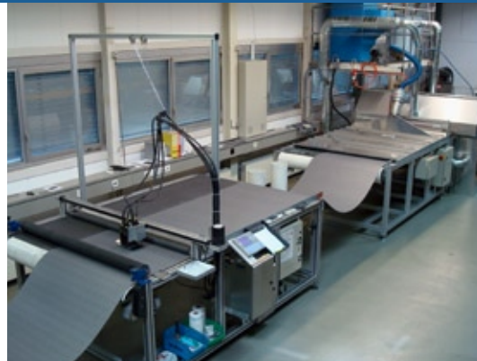
New anti-stick graphite coating line
