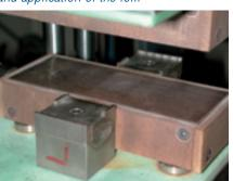
The following equipment is all you need to complete the weld: a grinder for preparing the joint; and two electrically heated plates and the KLINGER®-top-chem welding tape as welding compound (see pictures). The temperature of the plates must lie between 340 - 370 °C, and should not exceed 400 °C.
