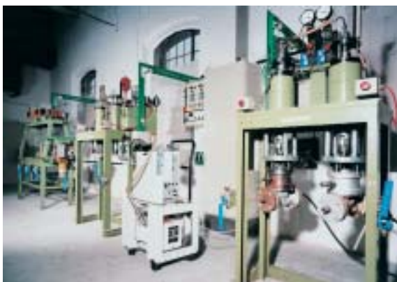
KVN KX1-GT 50.000 cycle test
