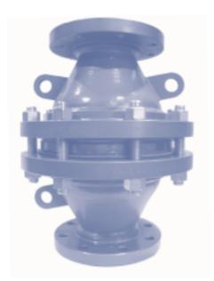
These units are specially designed for installation in pipeline applications with close proximity to the possible source of ignition, thereby confining the flame to the immediate area. Wherever a flammable gas or vapour is transported a flame arrester should be fitted to prevent the transmission of ignited flames which could cause a major incident, whilst allowing the process gas to flow under normal conditions.
